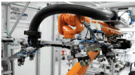
In the converted plant, injection-moulded parts made of glass fibre-reinforced polyamide with specially developed gripping technology are removed from an injection moulding machine and handled via the various stations. The hollow part consists of two halves for reasons of geometry. For further processing, the components are cooled down to room temperature via an active cooling section. The removed components are then joined, a metal filter is inserted and welded in the hot gas welding process.
