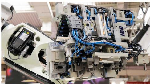
Multi-gripper for handling material
