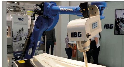
3D preform trimming with ultrasonic knife
